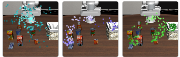
Fig. 9: Comparison of exploration behaviors on the task, “pick up the butter and put it in the basket” for RLPD (left), DSRL (center), and TMRL (right). TMRL leverages action sequences from smoothed contexts, resulting in broadened, yet coherent exploration.
