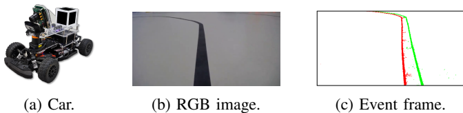
Fig. 3: (a) RoboRacer car equipped with Sony/Prophesee IMX636 sensor for the real-world deployment of the proposed algorithm. (b) RGB frame and (c) the corresponding DVS event frame representation.
